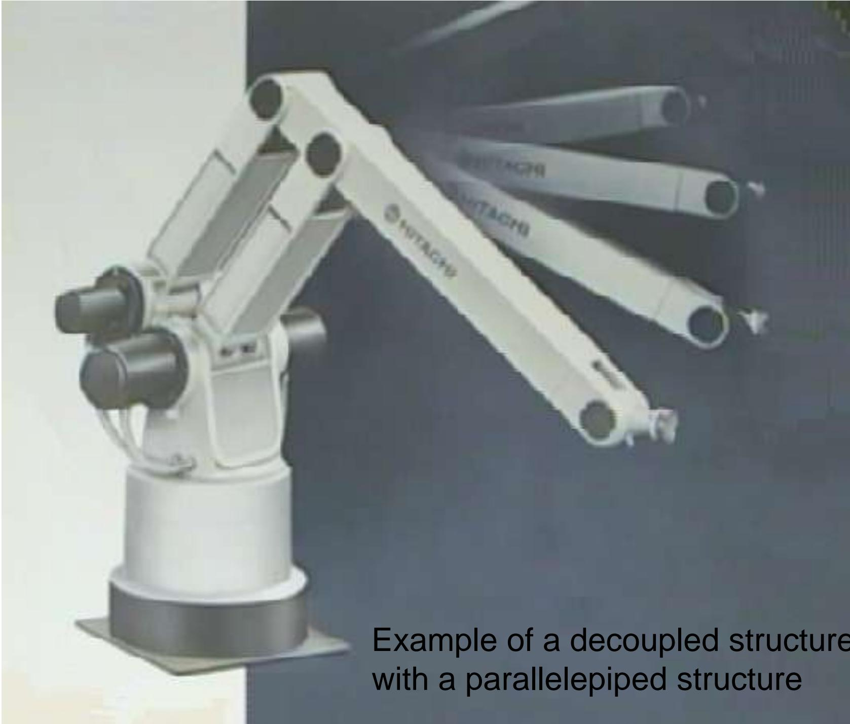
Example of a decoupled structure
