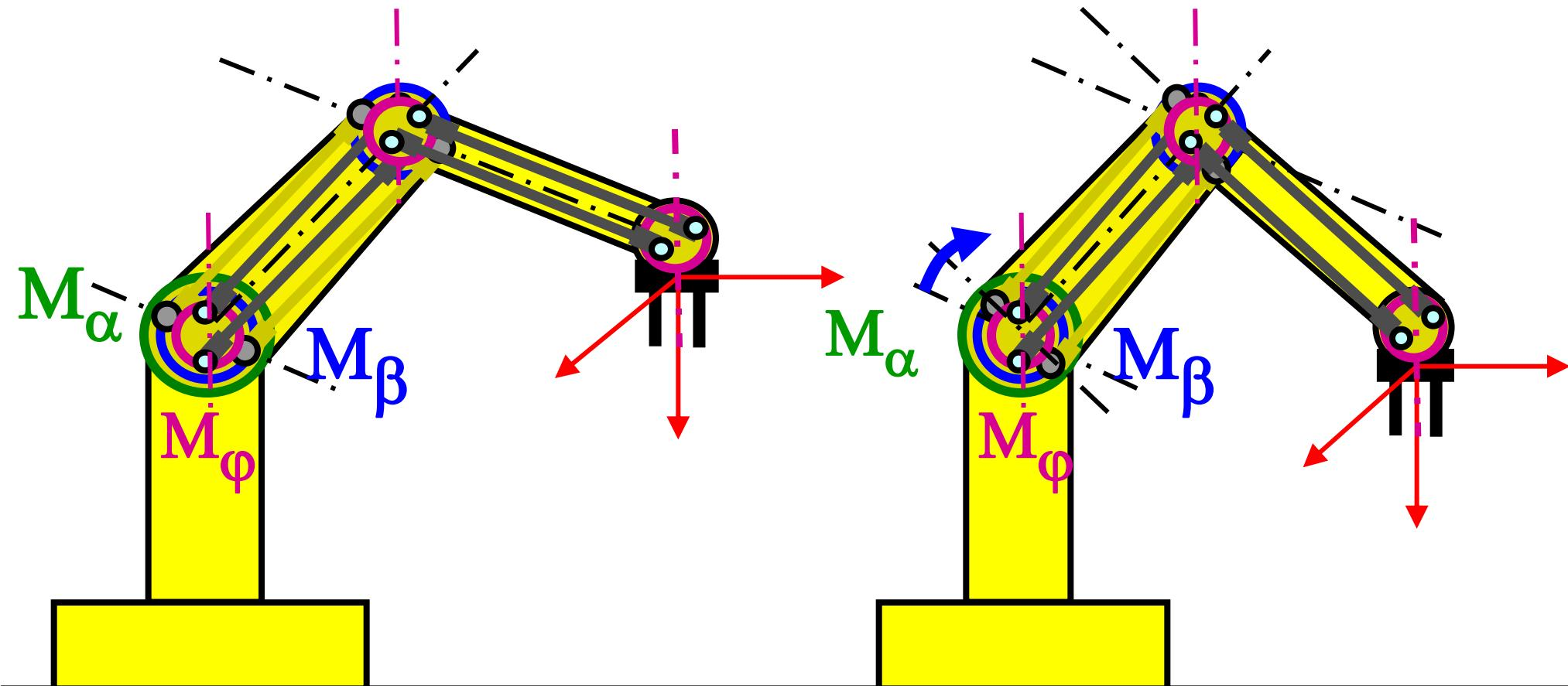
Transmission with connecting rods through two consecutive joints maintains the orientation of the E.E.
