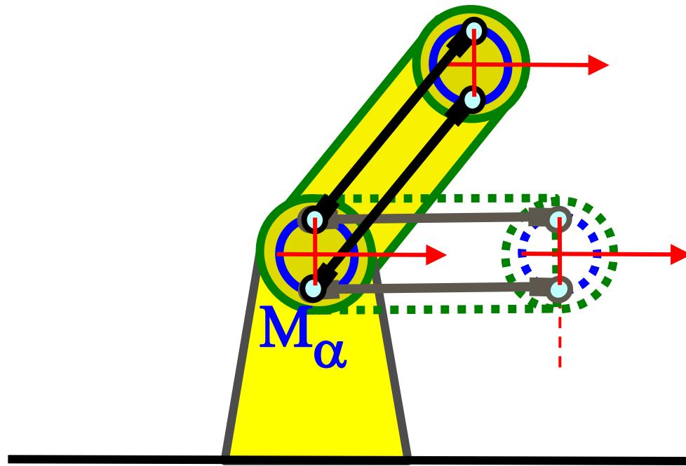
By transmitting the movement with connecting rods, the rotation of a joint does not propagate to the following.
