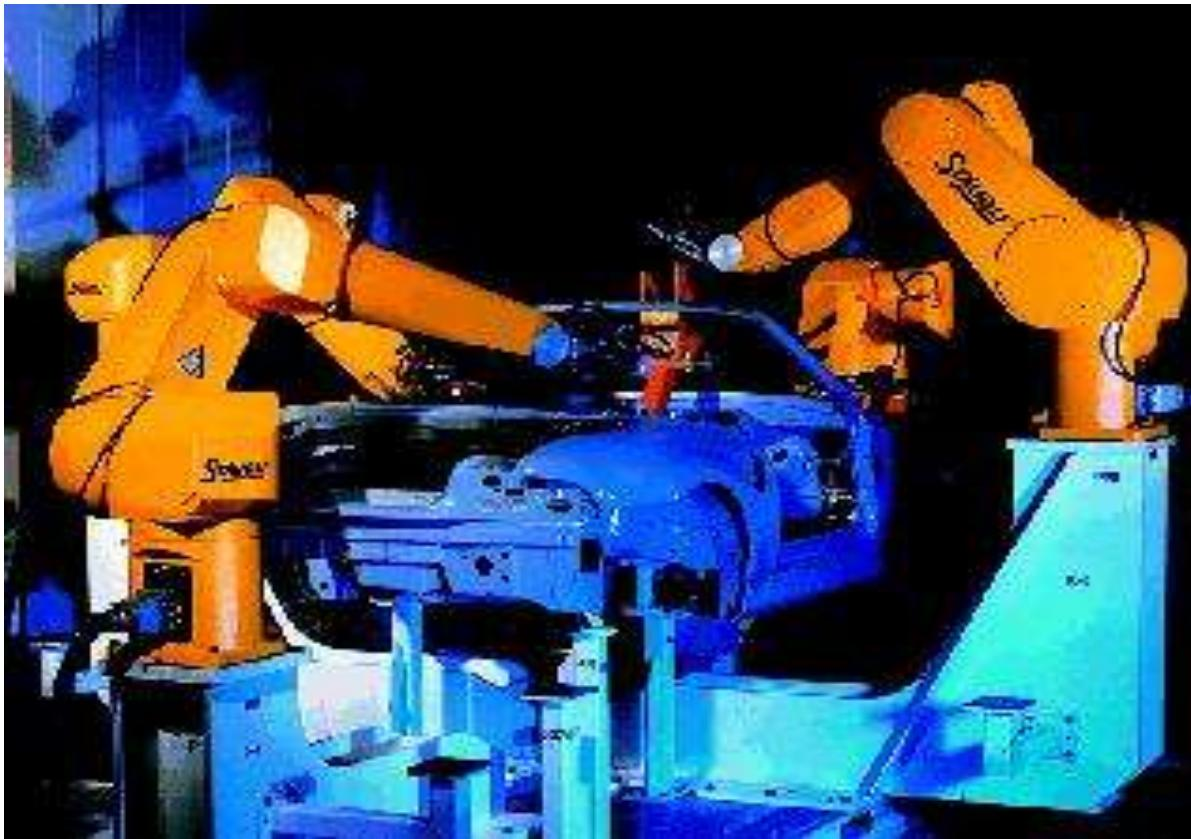
Example of Angular Work Space Robots (R+R+R)
