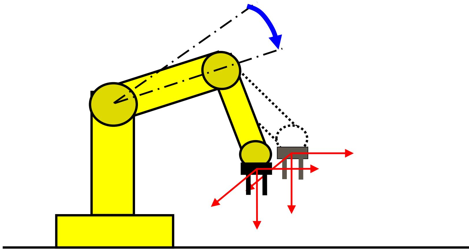
The rotation of a link is not propagated to the rest of the chain
