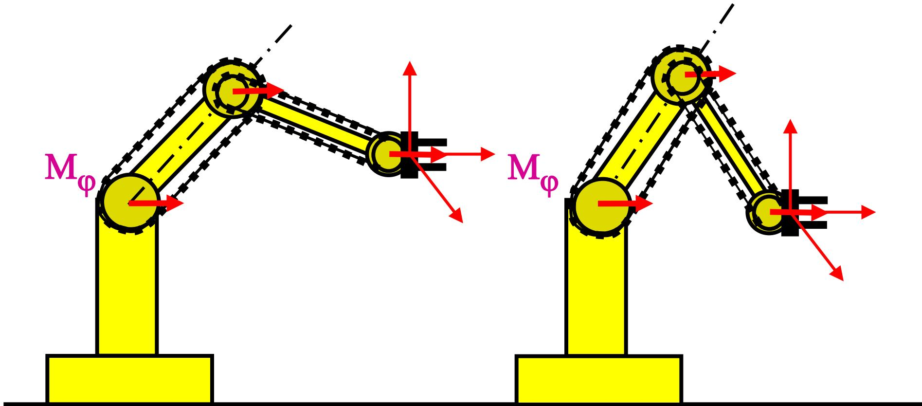
Transmission systems with chains produce decoupled movements
