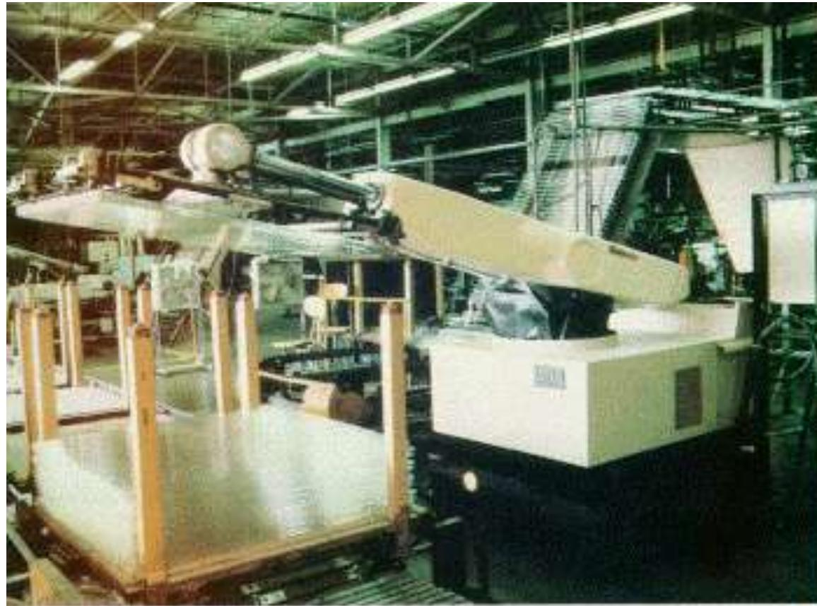
Example of a Polar Work Space Robot (R+R+D)
