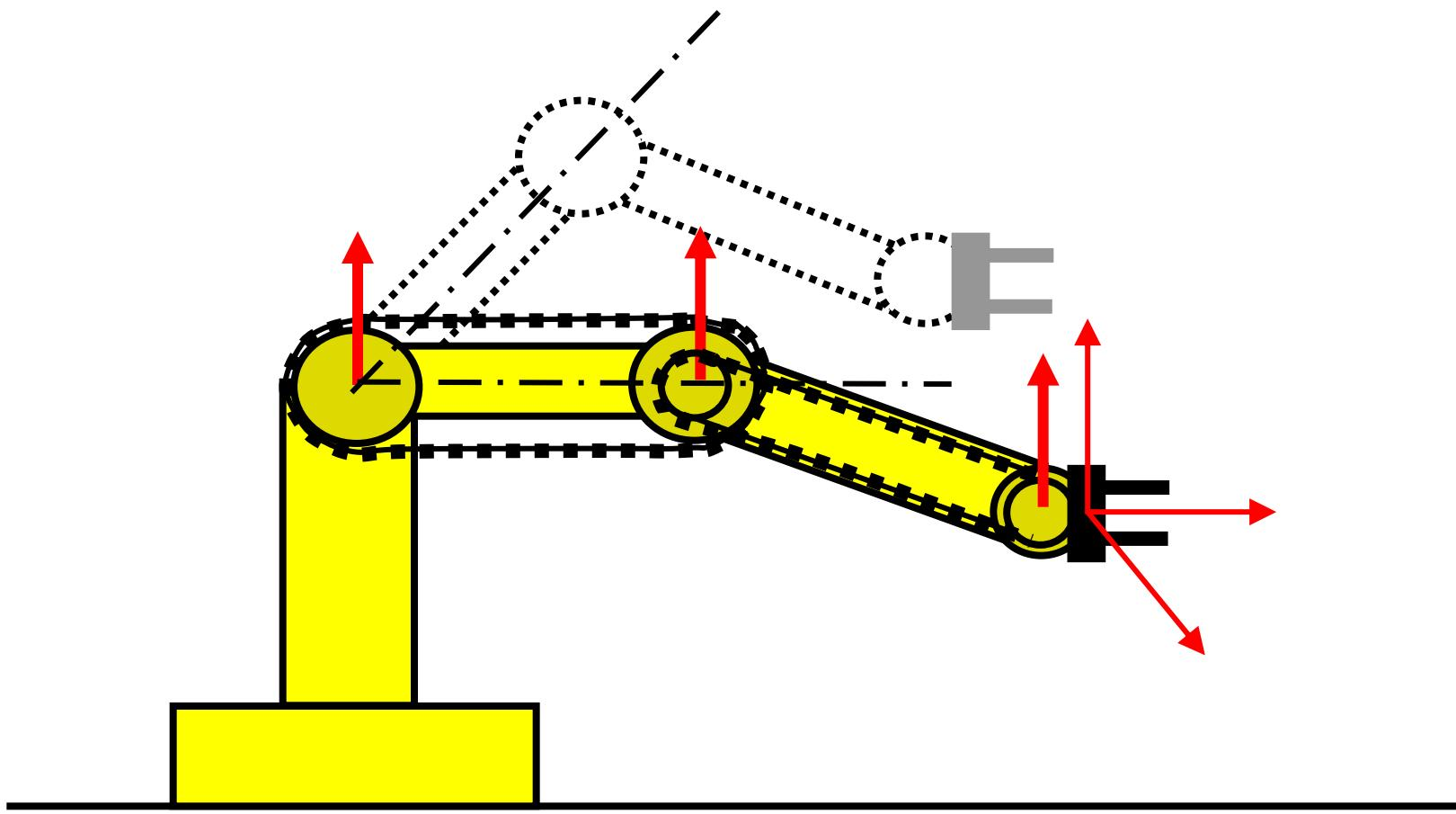
Structure decoupled with chains
