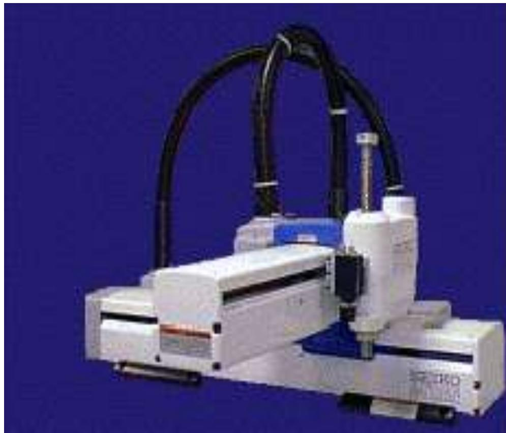
Example of a Cartesian Work Space Robot (D+D+D)
