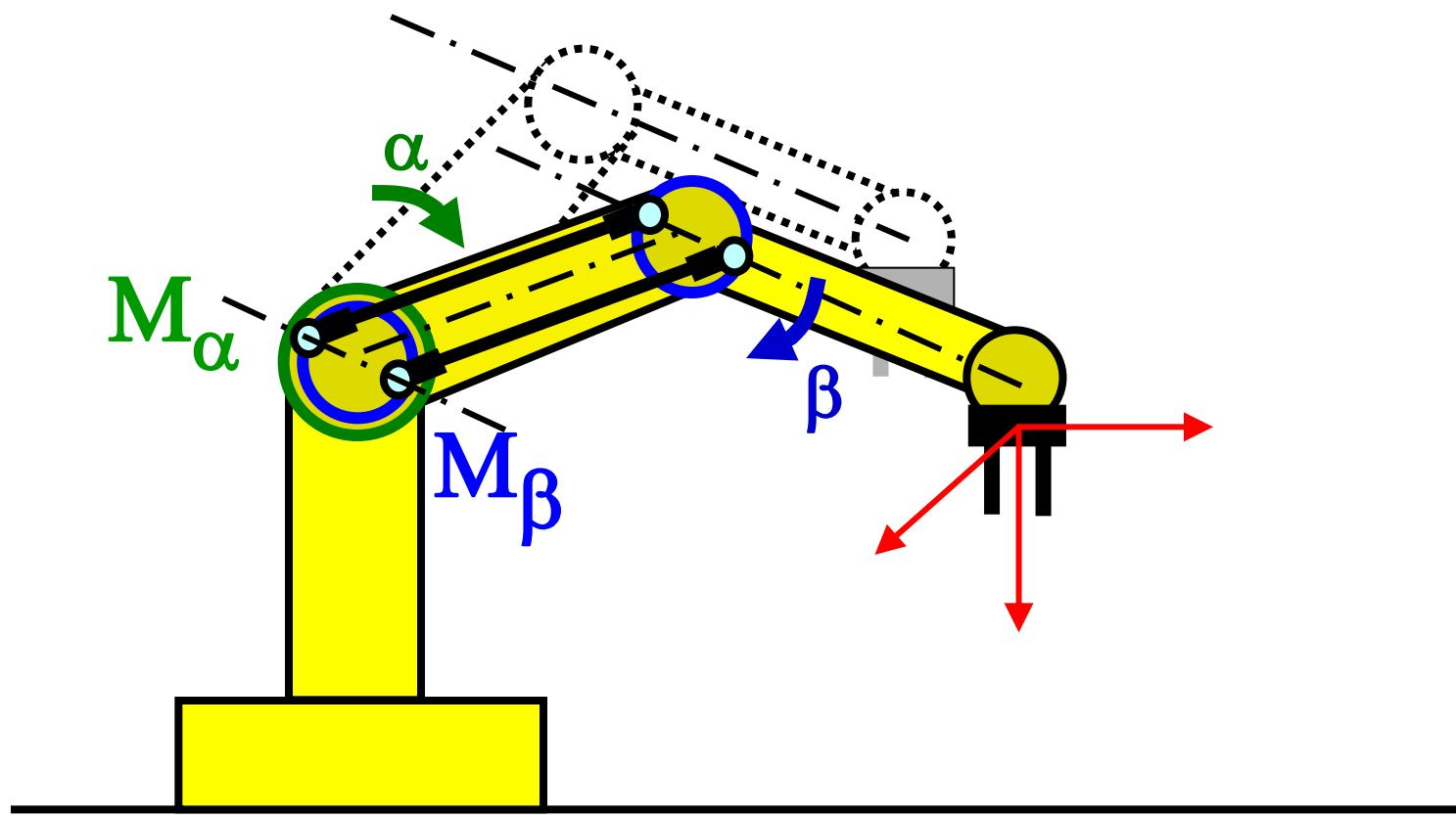
By transmitting the movement with connecting rods, the rotation of a joint does not propagate to the following.
