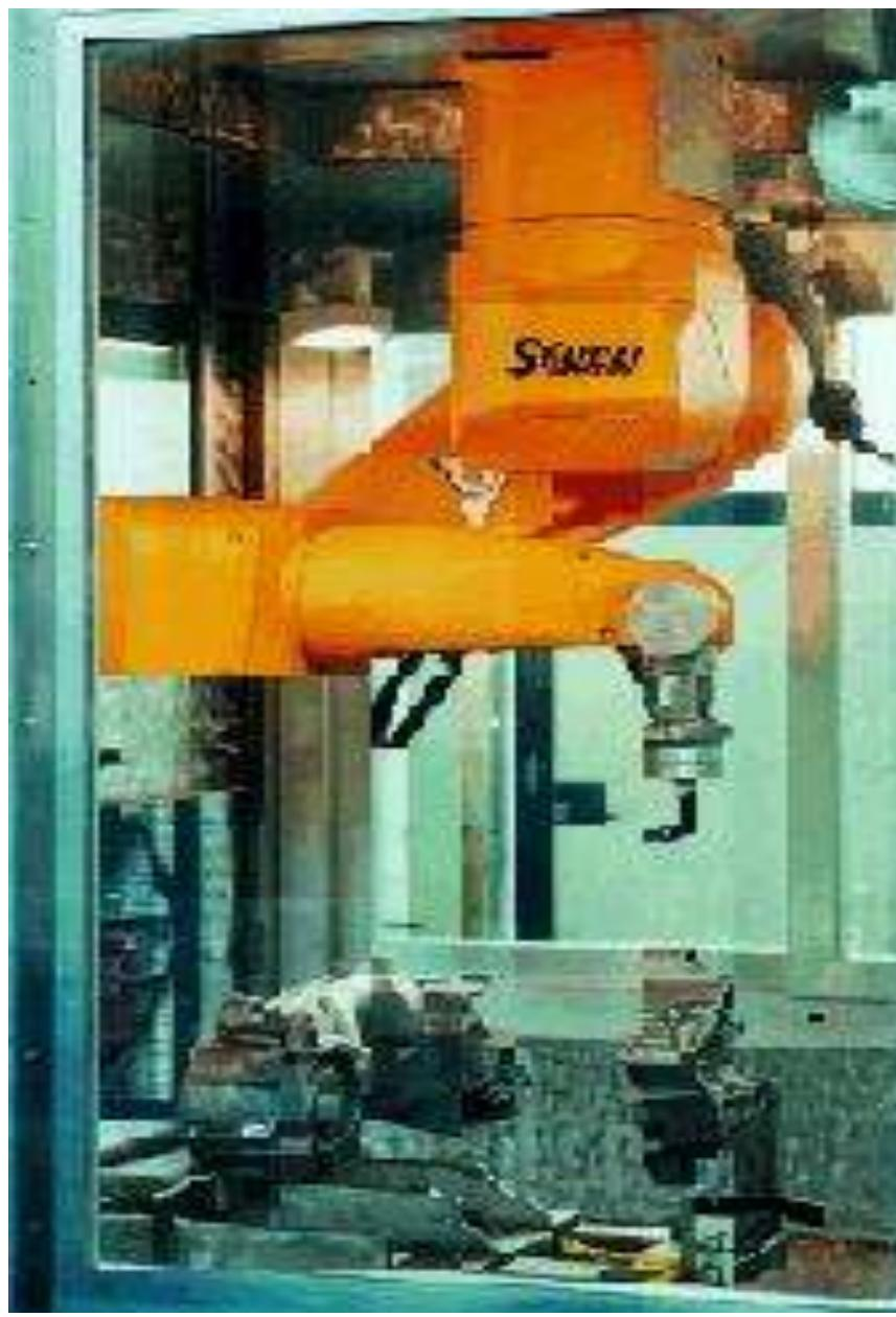
***Inverted robot: Increase the useful working volume***
