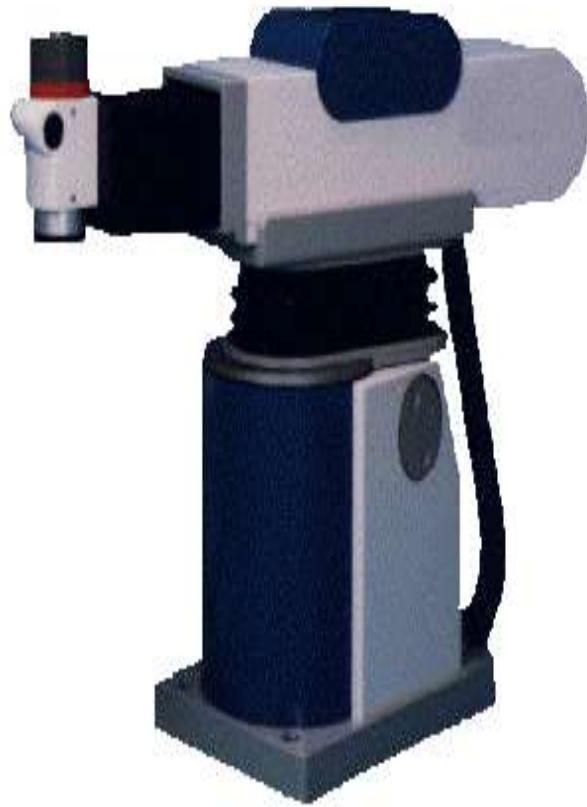
Example of a Cylindrical Work Space Robot (R+D+D)
