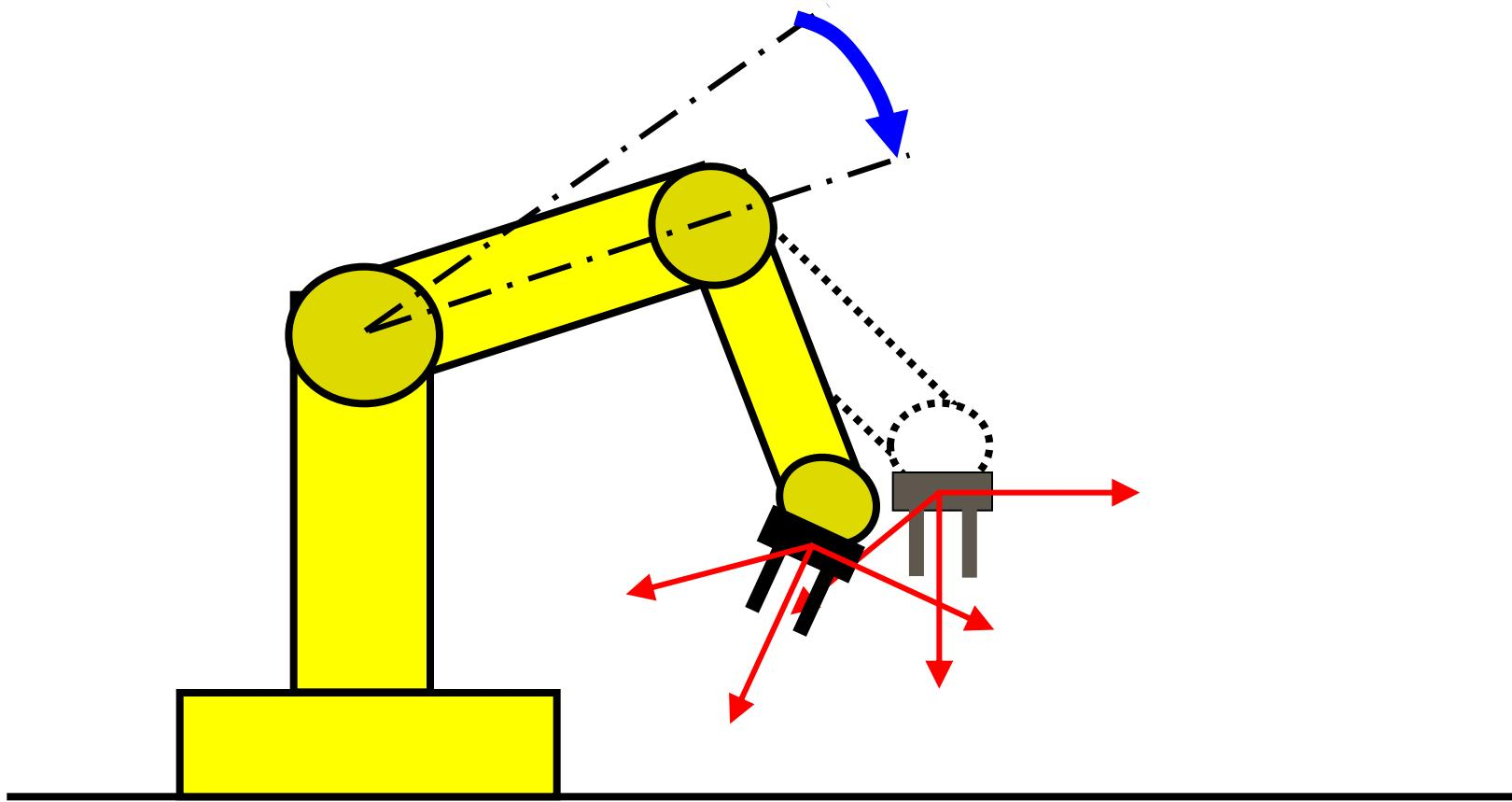
The rotation of a link is propagated to the rest of the chain
