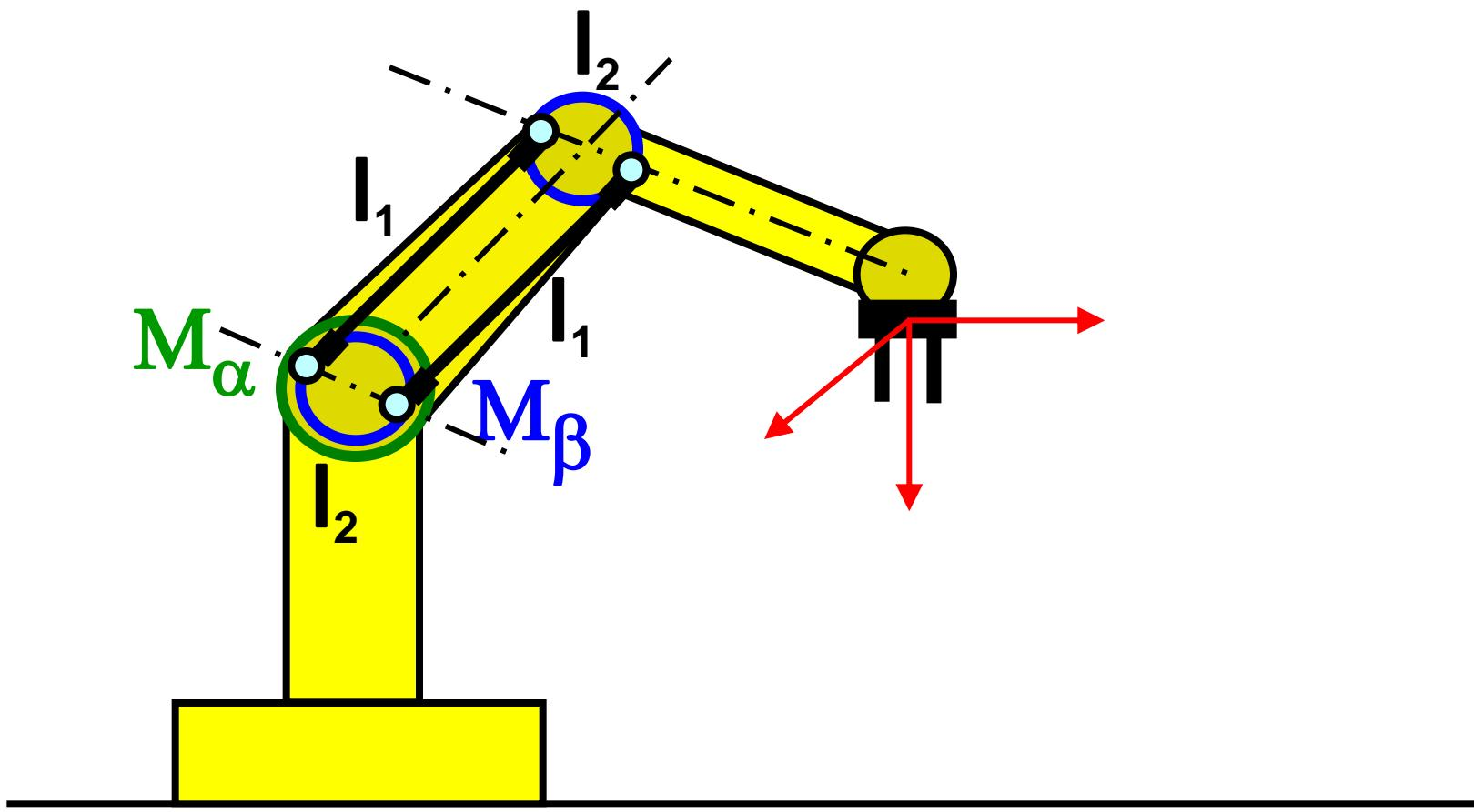
Structure decoupled with connecting rods
