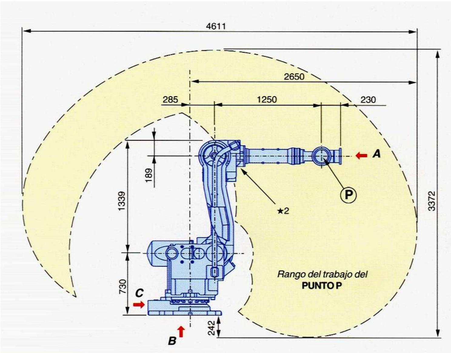
Working space of a robot with angular joints
